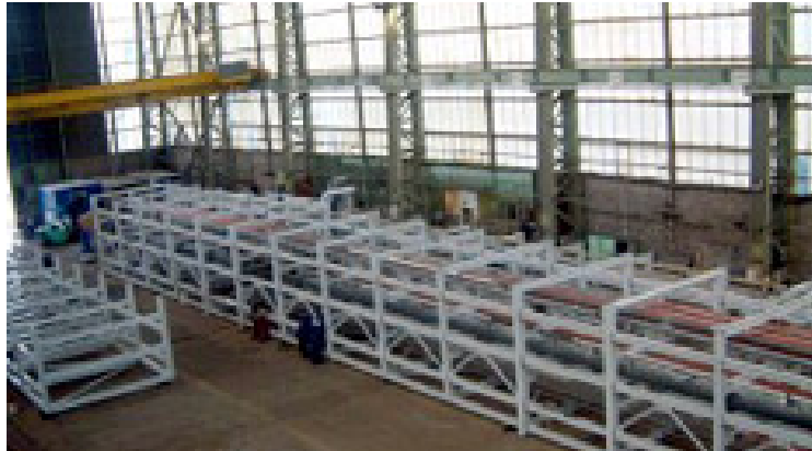
Figure 3 – Pre-fabricated and pre-loaded pipe racks prepared in a workshop
